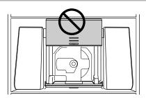
Place this unit in an area with more than 300 mm  $(11^{13}/_{16}")$  of vertical space.
